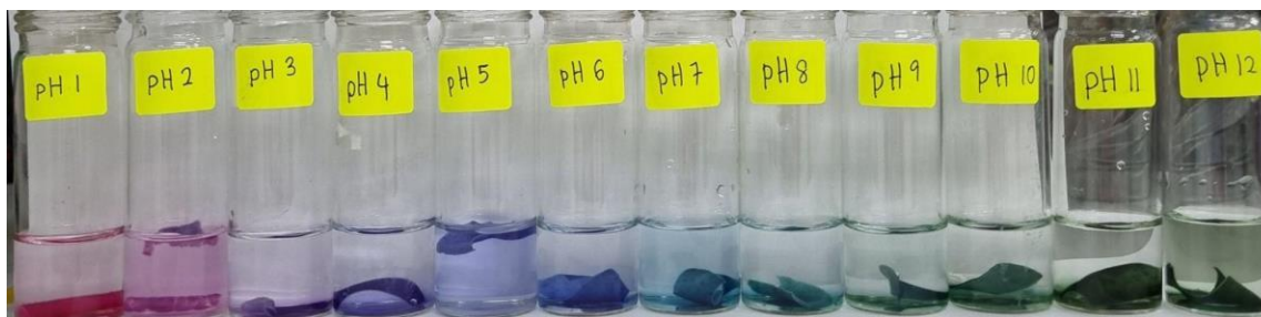
Figure 2. Colour response of Q/F-BPF 10% films in different pH buffer solutions (pH 1.0-12.0)
